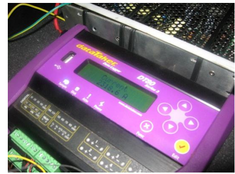
Figure 21 – The Load Box Controller Measured 2387 amps when the Sensor System Measured 2318.6 amps
