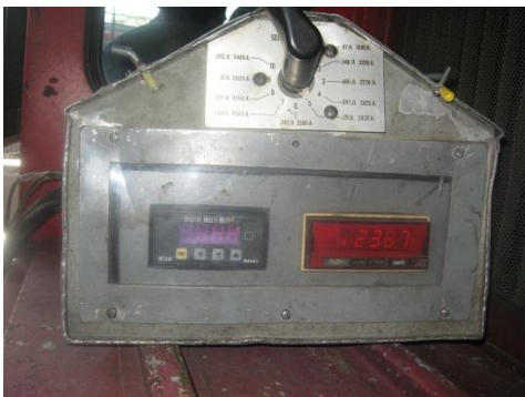
Figure 21 – The Load Box Controller Measured 2387 amps when the Sensor System Measured 2318.6 amps
