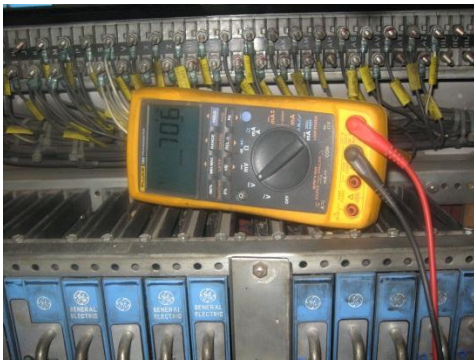
Figure 20 – A Handheld Voltmeter Measured 706 volts when the Sensor System Measured 708.8 volts
