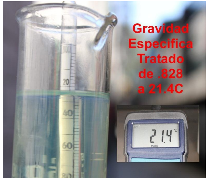
Figure 13 – FPC Treated Fuel Specific Gravity Measurement
