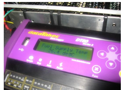
Figure 22 – A Handheld Digital Thermometer Measured 26.4°C when the Sensor System Measured 26.4°C for the Fuel Supply Temperature
