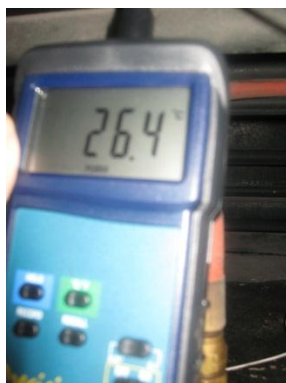
Figure 22 – A Handheld Digital Thermometer Measured 26.4°C when the Sensor System Measured 26.4°C for the Fuel Supply Temperature
