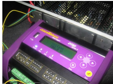
Figure 20 – A Handheld Voltmeter Measured 706 volts when the Sensor System Measured 708.8 volts
