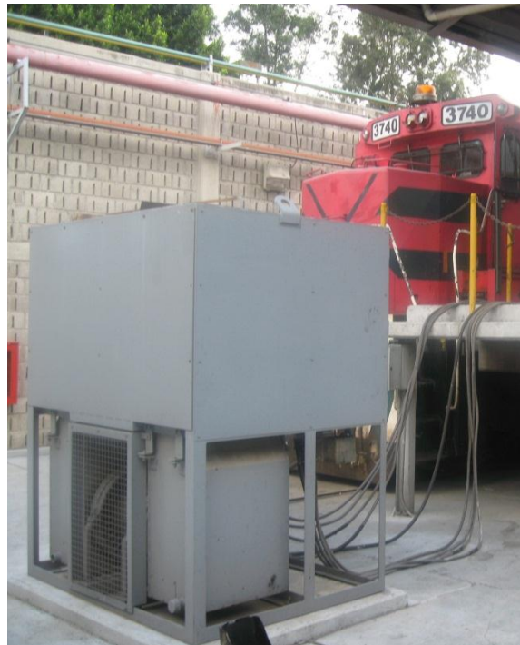
Figure 8 – Load Box Connected to Test Locomotive
